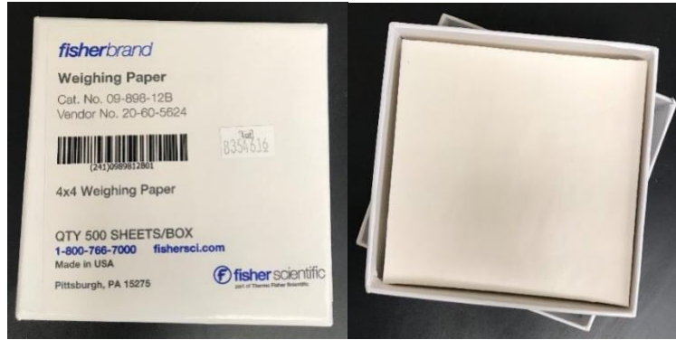
Figure 2: Example of weighing paper for C14 “dust” collection.
