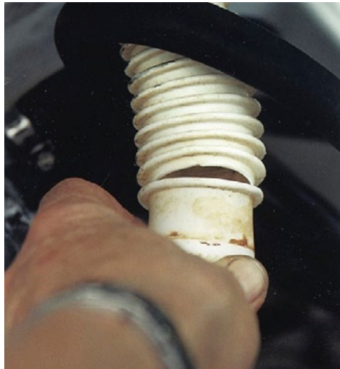
Checking hoses are an important part of spring commissioning Photo credit: BoatUS.
