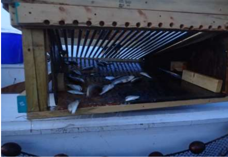
Figure 4. Fish culling table separating small fish from catch and channeled back into the water alive.
