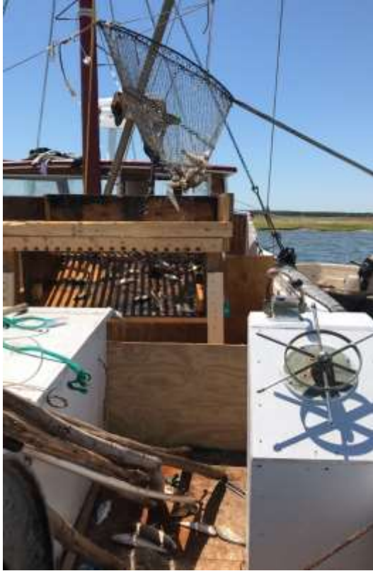
Figure 2. Fish brailled from seine pocket onto culling table on boat deck.
