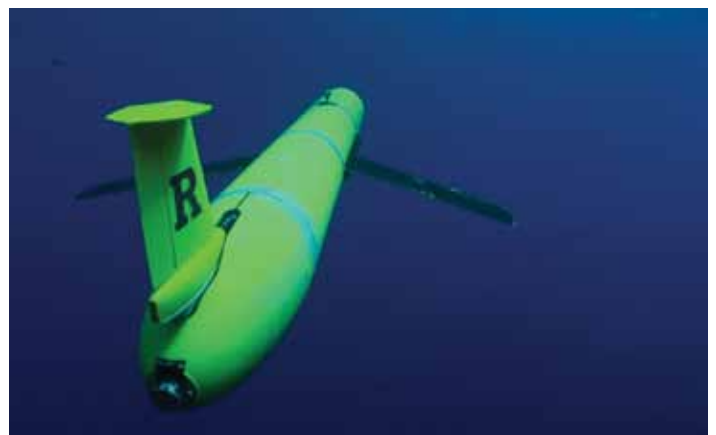
Figure 3. Rutgers University's autonomous glider, RU 27 nicknamed the Scarlet Knight, completed its 221 day and 7,409 mile journey from New Jersey to Baiona, Spain.
