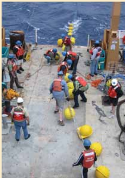
Figure 2. Scientists and technicians deploy Stratus X buoy in 4440m (over 2.75 miles) of water off the coast of Chile, where a deck of stratus clouds make sea surface measurements from satellite impossible. The importance of teamwork and safety can not be overestimated.
