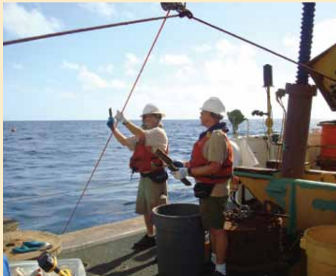
Figure 7. Rick and Art place fairings on the Nielspin (a plastic coated conductive wire) to help reduce drag on the anchor line from strong currents at the Equator. (A. Bangert)
