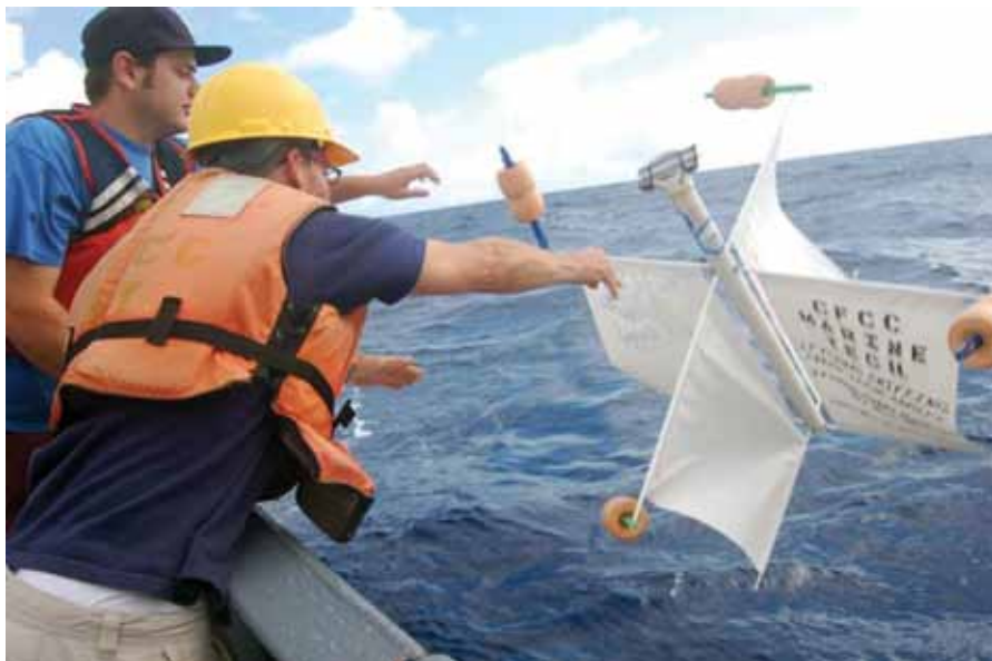
Students from Cape Fear Community College of Wilmington, NC launch a drifter that collects real-time information about ocean currents.
